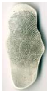
Figure 5 White silicone lift from textured surface (computer)
